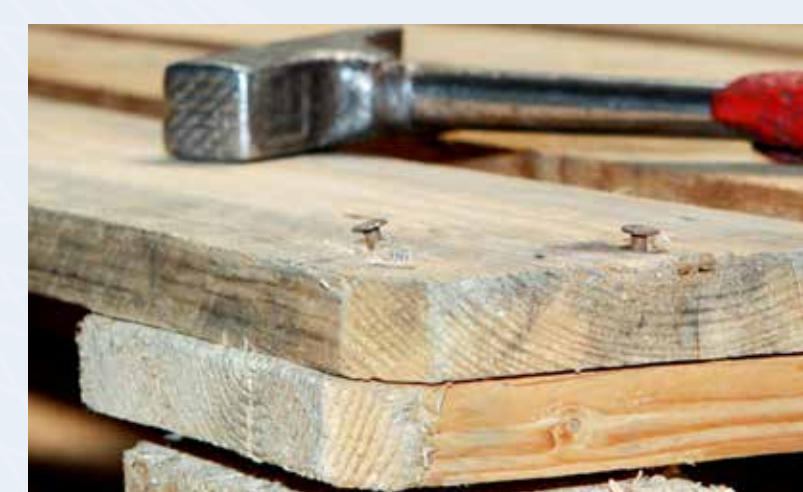
Hammering down projecting fastening elements
